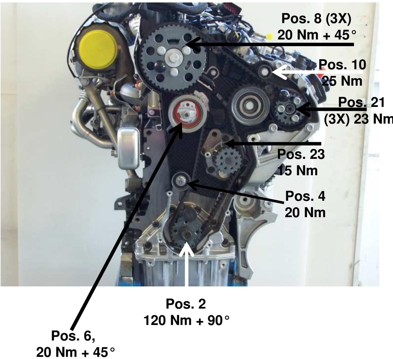
**Pos. 2 Screw for the crankshaft pulley:**
